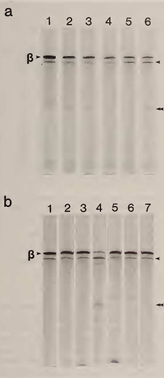
FIG. 3. Hydrolysis of isolated \beta -connectin by calcium-activated neutral protease. \beta -Connectin, 0.5 mg/ml was incubated with CANP, 1:20 by weight ratio, in 0.3 M NaCl and 20 mM Tris buffer, pH 7.5, at 25^\circ\text{C} . a, time course in the presence of 3 mM \text{CaCl}_2 . 1, 0 time; 2, 1 min; 3, 2 min; 4, 10 min; 5, 30 min; 6, 60 min. b, effects of various agents. Incubated for 30 min. 1, initial; 2, control after incubation; 3, CANP; 4, CANP+3 mM \text{CaCl}_2 ; 5, CANP+3 mM \text{CaCl}_2 +1 mM E64c; 6, 3 mM \text{CaCl}_2 +1 mM E64c; 7, 3 mM \text{CaCl}_2 . \beta , \beta -connectin; arrowheads, 1700 kDa peptide; double arrowheads, 400 kDa peptide.
